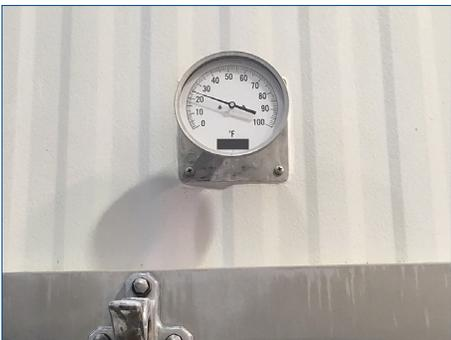
To meet USDA requirements, the temperature measurement device in this application must have an accuracy of at least  $\pm 1^\circ\text{F}$ . The processor was previously using a five inch dial bimetal thermometer – large enough to read the temperature across the room.
